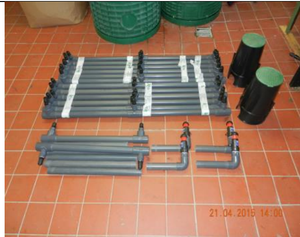
Pre-assembled PVC manifolds and air vents
